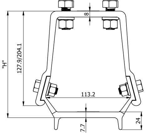
NOTE: MATERIAL: ALUMINIUM ALLOY HARDWARE: GALVANIZED STEEL ACCESSORIES: TWO HEX NUTS, SINGLE COIL LOCK WASHER & BOLTS 1/2"x30mm TWO HEX NUTS, SINGLE COIL LOCK WASHER & BOLTS 3/8"x25mm.
